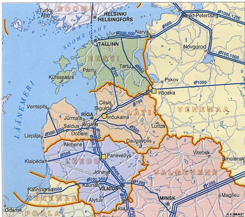
Figure 2. Gas pipelines in the Baltic States.
