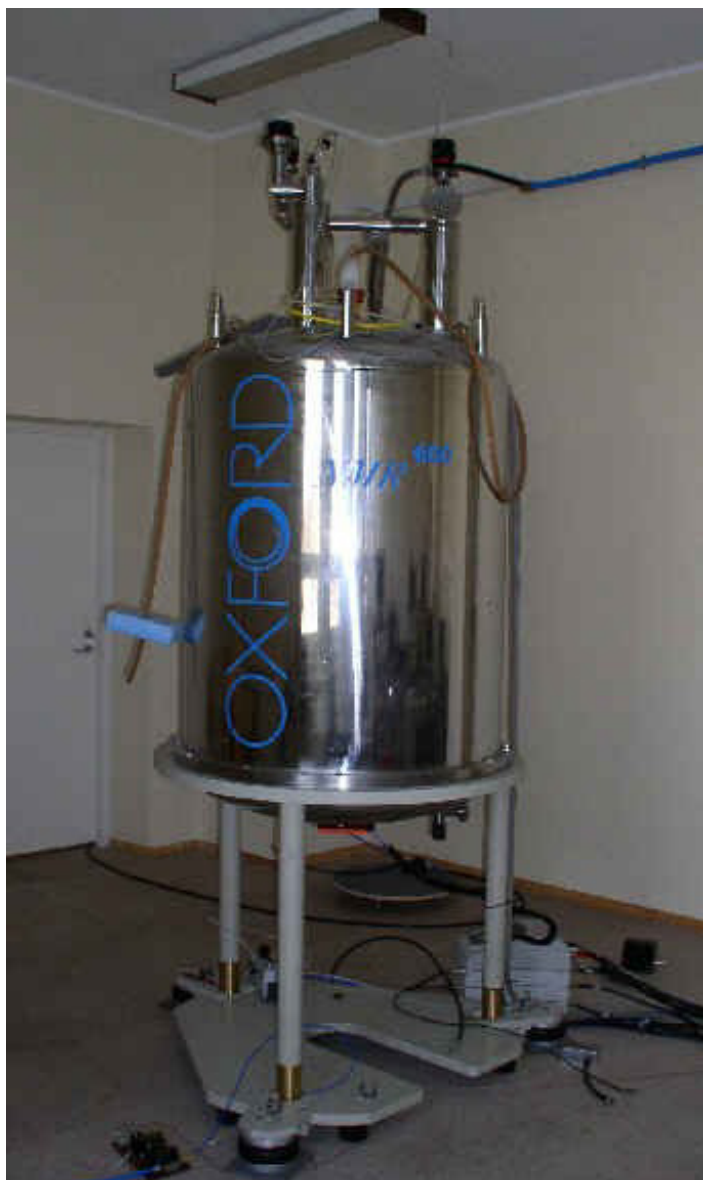
The new Oxford Instruments superconducting magnet of the 600 MHz 2D-FT-NMR spectrometer.
