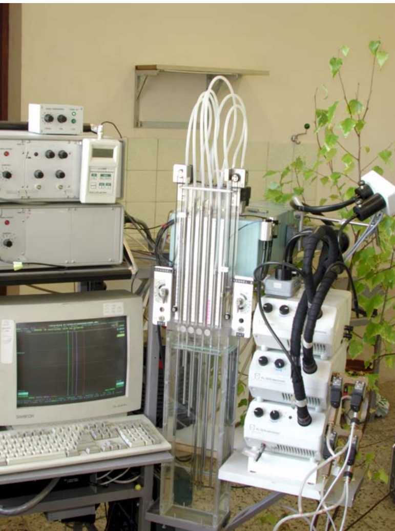
An apparatus for the investigation of leaf photosynthesis using gas exchange and optical methods.
